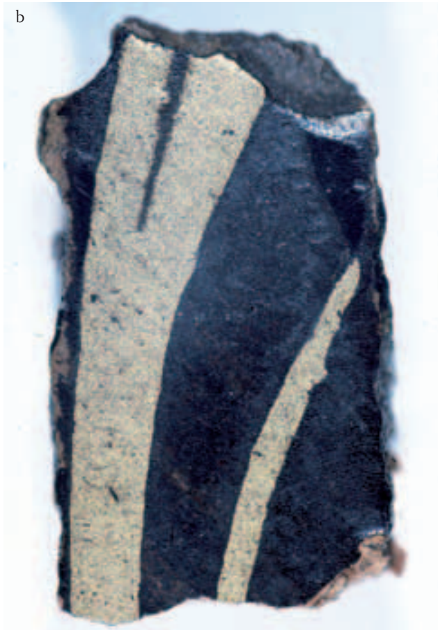
Figure 7 The Mazarin Chest: (a) SEM image at \times 1000 magnification of scrolling hiramaki-e decoration from the border, lid exterior. Image courtesy of the V&A and N. Hayakawa of the National Research Institute of Cultural Properties, Tokyo. (b) Macro photograph of a flake from the scrolling border of the lid exterior showing loss of small areas of hiramaki-e decoration. Macro photograph: Y. Yamashita, courtesy of the V&A.
