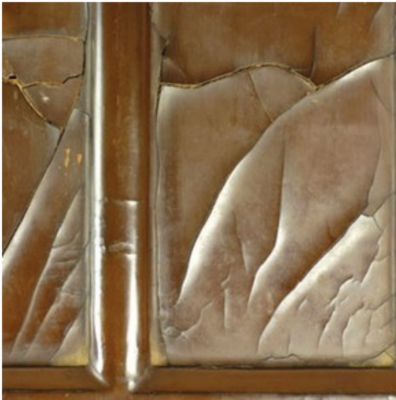
Figure 2. FE.7-1973 Detail of a Chinese lacquer cabinet showing extensive cracking of the lacquer coating on the inside of the drop-front (Photography by Nanke Schellmann) (click image for larger version)
