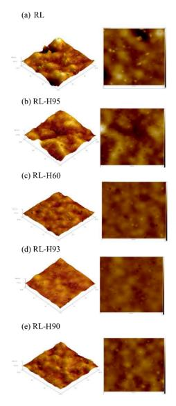
**Figure 4.** Atomic force microscope (AFM) analysis of RL films with different HALS additives (**a**) RL (**b**) RL-H95 (**c**) RL-H60 (**d**) RL-93 (**e**) RL-H90.
