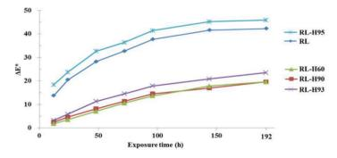
**Figure 1.** Time dependent color difference ( $\Delta E^*$ ) of RL films with different HALS additives. **Table 2.** Lightfastness of RL films with different HALS additives after 192 h UV exposure test.
