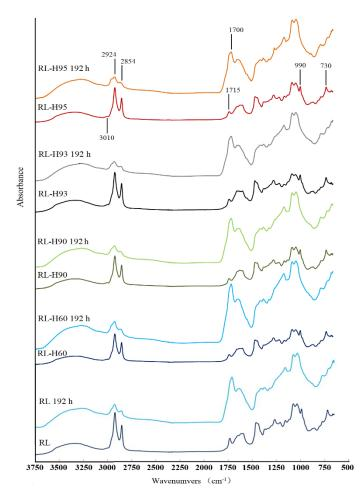
Figure 3. Fourier transform infrared spectroscopy (FTIR) spectra of RL films with different HALS additives.
