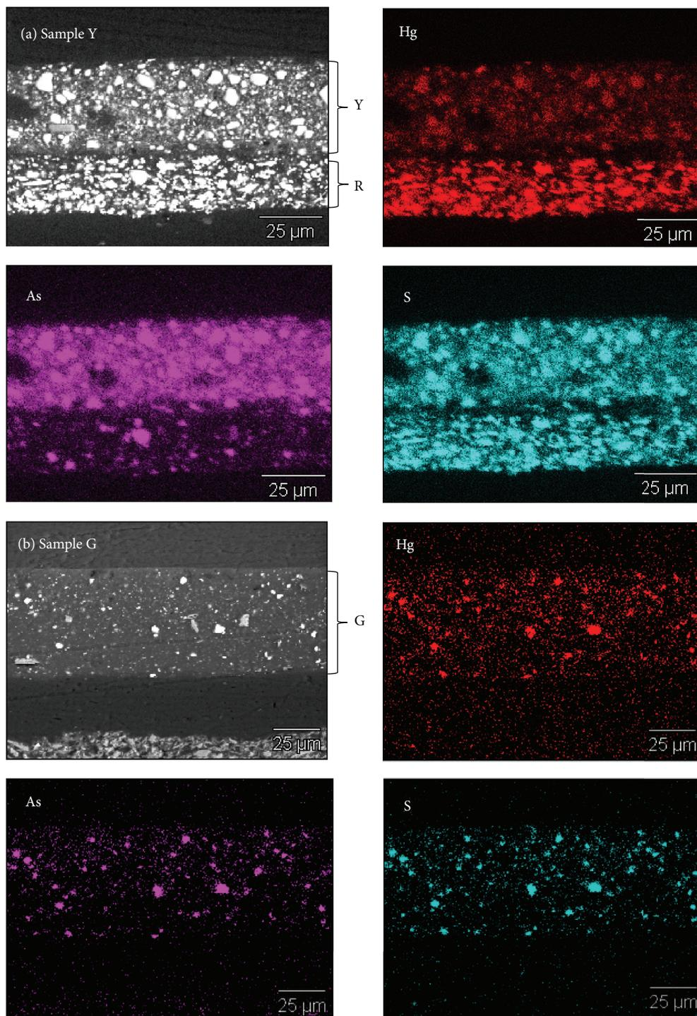
FIGURE 5: Cross-sectional element mapping experiments. (a) Sample Y, (b) Sample G.
