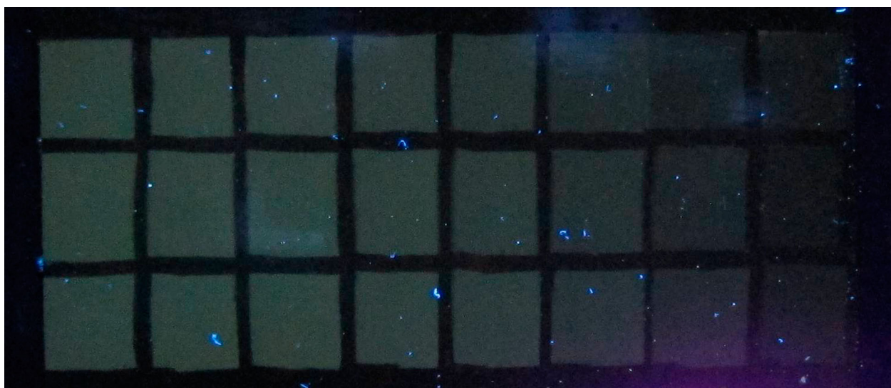
Figure 9 Black urushi with oil added (sample U4), observed under ultraviolet light after 12 hours light exposure in 30-minute increments at 0.33 \text{ W m}^{-2} . Exposure increases from top left to bottom right.
