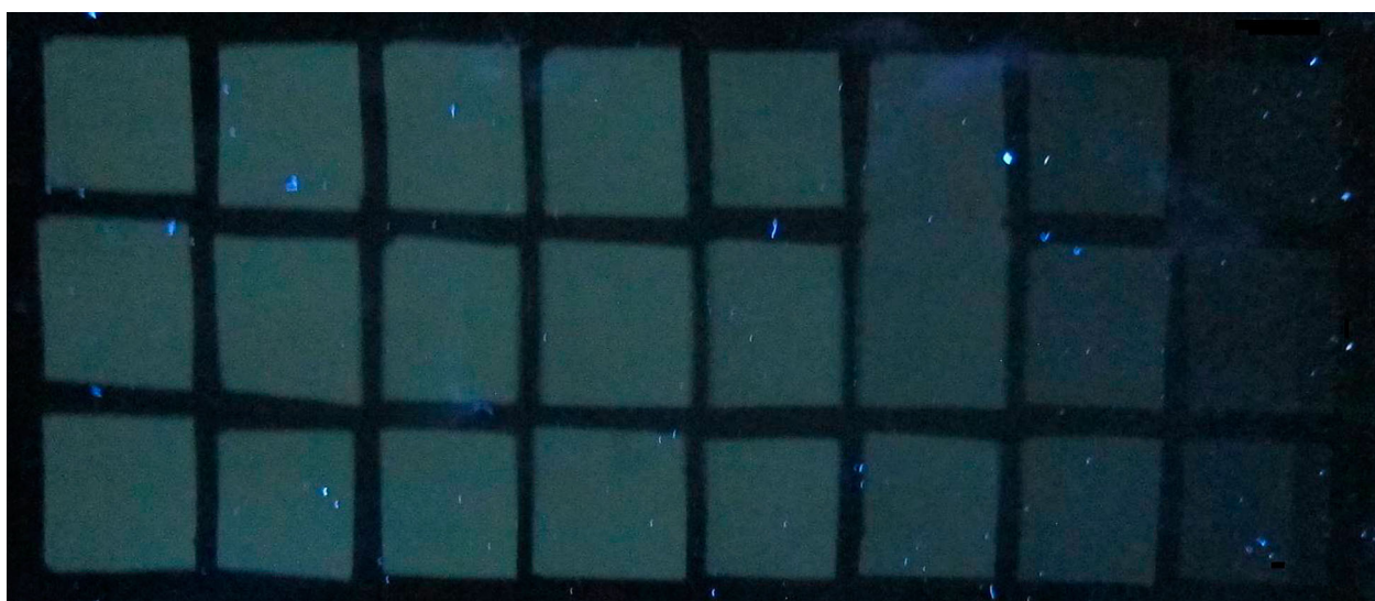
Figure 10 Black laccol with oil added (sample L2), observed under ultraviolet light after 12 hours light exposure in 30-minute increments at 0.33 \text{ W m}^{-2} . Exposure increases from top left to bottom right.
