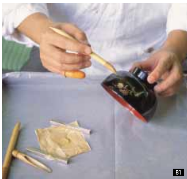
78. Applying a strip of cloth to the edges of a wooden bowl with urushi .
