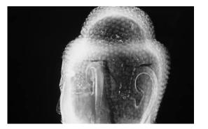
Fig. 7.18. Amida sculpture (B6oS10+), X-radiograph of head, side view. Technical data: Gulmay X-ray unit (320 kV max.), Kodak Industrex AA film, 35 kV, 5 mA, 60 seconds, distance from tube, 36 inches.
