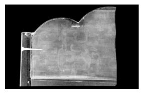
Fig. 6.28. X-ray of cresting rail on lacquer chair (B69M54a), showing use of handmade ferrous nails. Technical data: Norelco X-ray unit (150 kV max.), Kodak Industrex AA film, 45 kV, 5 mA, 120 seconds, distance from tube, 36 inches.
