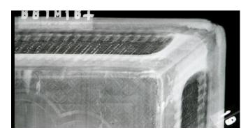
Fig. 5.33. Box (B61M16+), X-radiograph of lid corner; note the absence of dowels or nails in the joins and the way in which the basketry is applied as a band that wraps around the corner Technical data: Gulmay X-ray unit (320 kV max.), Kodak Industrex M film, 30 kV, 4 mA, 60 seconds, distance from tube , 36 inches.
