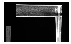
Fig. 6.32. X radiograph of arm on lacquer chair (B69M54a), showing attachment using a modern 3 1/2-inch screw. Technical data: Norelco X-ray unit (150 kV max.), Kodak Industrex AA film, 50 kV, 5 mA, 120 seconds, distance from tube, 36 inches.
