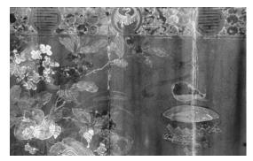
Fig. 8.7. X-radiograph of screen (B69M52), showing bamboo dowels and radio-opaque putty. Technical data: Norelco X-ray unit (150 kV max.); Kodak Industrex AA film; 40 kV, 5 mA, 30 seconds; distance from tube, 36 inches.
