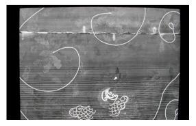
Fig. 6.18. Cabinet (B65M31), X-radiograph of lid; note discontinuous nail holes along join in wood. Technical data: Gulmay X-ray unit (320 kV max.), Kodak Industrex AA film, 25 kV, 5 mA, 60 seconds, distance from tube, 36 inches.
