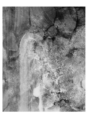
Fig. 7.42. Head of a Bodhisattva (B6oS14+); X-radiograph showing vertical seam remaining from fabrication in two-part mold. Technical data: Norelco X-ray unit (150 kV max.), Kodak Industrex M film, 35 kV, 4 mA, 90 seconds, distance from tube, 36 inches.
