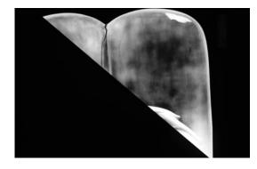
Fig. 7.34. Helmet (B87M22a), X-radiograph of laminated paper superstructure. Technical data: Norelco X-ray unit (150 kV max.), Kodak Industrex AA film, 40 kV, 6 mA, 60 seconds, distance from tube, 36 inches.
