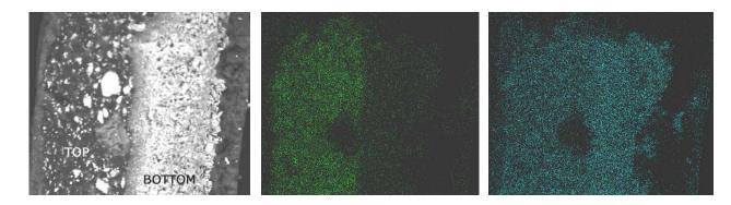
Fig. 8.12. X-radiograph dot maps of red pigment for lead and for mercury; dot maps for iron and cadmium were unremarkable.
