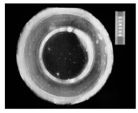
Fig. 4.03. X-radiograph of bowl (B65M26). Technical data: Norelco X-ray unit (150 kV max.), Kodak Industrex M film, 40 kV, 4 mA, 90 seconds, distance from tube, 36 inches.
