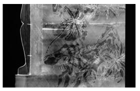
Fig. 8.19. X-radiograph, screen (B67M8+). Technical data: Norelco X-ray unit (150 kV max.); Kodax Industrex AA film; 45 kV, 5 mA, 60 seconds; distance from tube, 36 inches.
