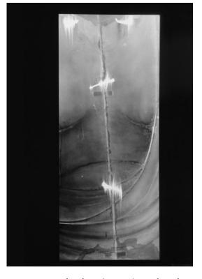
Fig. 7.15. Amida sculpture (B6oS10+), X-radiograph of front of torso. Technical data: Gulmay X-ray unit (320 kV max.), Kodak Industrex AA film, 25 kV, 5 mA, 60 seconds, distance from tube, 36 inches.
