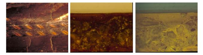
Fig. 4.25. Tray (B60M164), photomicrograph show-ing wire structure.
