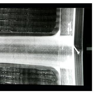
Fig. 5.29. Box (B61M16+), X-radiograph of base corner; the more radio-opaque areas framing the basketry are the wood strips that secure the basketry to the box; joins in these strips are visible near the corner and the image also shows the use of wire nails applied from interior and exterior of box. Technical data: Gulmay X-ray unit (320 kV max.), Kodak Industrex M film, 30 kV, 4 mA, 60 seconds, distance from tube, 36 inches.
