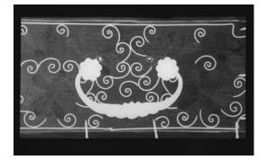
Fig. 6.16. Cabinet (B65M31), X-radiograph of drawer front; note presence of metal in holes for an earlier handle and current use of wire nails in the joins. Technical data: Gulmay X-ray unit (320 kV max.), Kodak Industrex AA film, 25 kV, 5 mA, 60 seconds, distance from tube, 36 inches.
