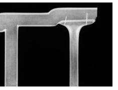
Fig. 6.31. X radiograph of arm on lacquer chair (B69M54a); note fineness of decoration. Technical data: Norelco X-ray unit (150 kV max.), Kodak Industrex AA film, 45 kV, 5 mA, 120 seconds, distance from tube, 36 inches.
