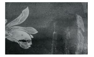
Fig. 8.8. X-radiograph of screen (B69M52), showing filled holes along edge for old hinges. Technical data: Norelco X-ray unit (150 kV max.); Kodak Industrex AA film; 40 kV, 5 mA, 30 seconds; distance from tube, 36 inches.
