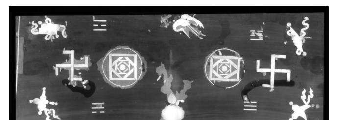
Fig. 6.6. X-radiograph of lid, Box (B60M292); large (1-cm diameter) insect tunnels are visible, as are lacquer repairs, particularly at center. Technical data: Norelco X-ray unit (150 kV max.), Kodak Industrex M film, 35 kV, 4 mA, 90 seconds, distance from tube, 36 inches.
