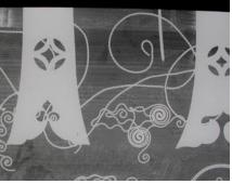
Fig. 6.19. Cabinet (B65M31), X-radiograph of large door; note discontinuous nail holes along wood joins and current use of wire nails in these joins. Technical data: Gulmay X-ray unit (320 kV max.), Kodak Industrex AA film, 25 kV, 5 mA, 60 seconds, distance from
