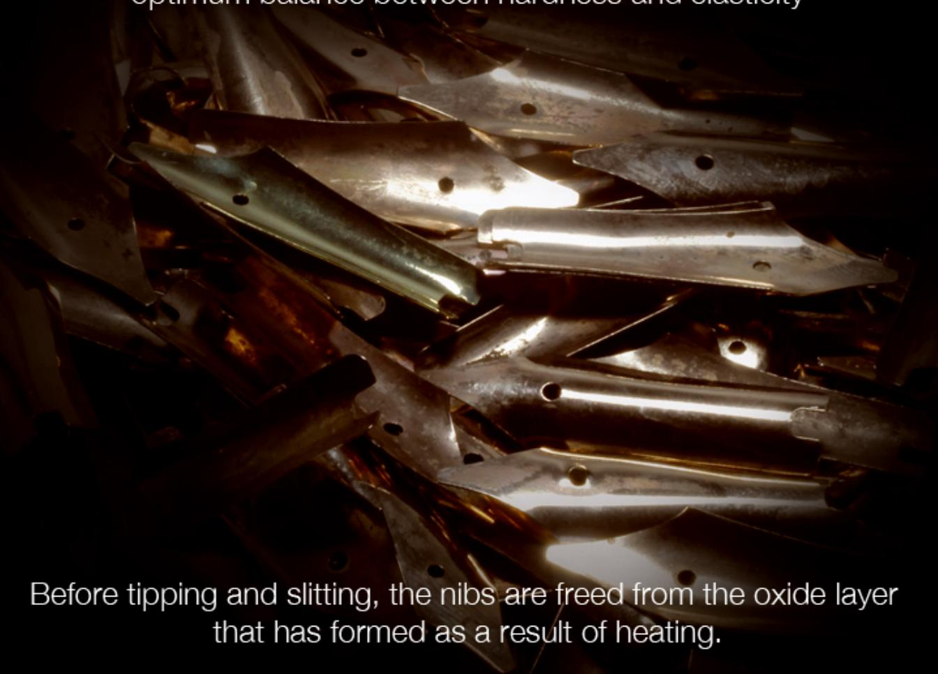
Before tipping and slitting, the nibs are freed from the oxide layer that has formed as a result of heating.
